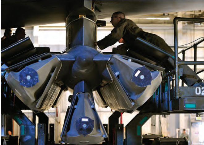
A pod of cruise missiles being loaded onto a B-52. The B-52 can carry up to 20 nuclear-armed cruise missiles. (Photo: U.S. Air Force)
