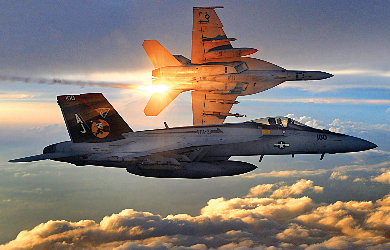
The U.S. Navy's FA-18 Hornet is designed to be both a fighter plane and a ground attack aircraft. Its versatility allows it to operate from aircraft carriers or land bases. The Hornet is capable of carrying the B61 thermonuclear bomb. The upgraded Super Hornet (shown here), though not designed to carry the B61, is bigger, can carry more munitions, and can fly much farther. (Photo: Open Source)
