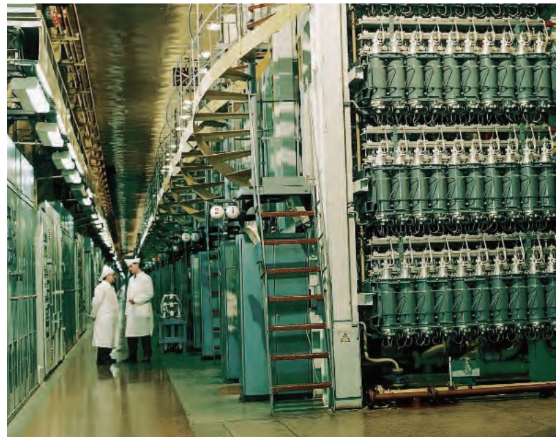
Surprise! Undetected by the U.S. intelligence community, by the mid-1980s the Soviet Union had converted its gaseous-diffusion technology for making highly enriched uranium to the highly efficient gas-centrifuge technology. The centrifuges (shown here) had doubled Soviet production capacity. (Photo: Open Source)
