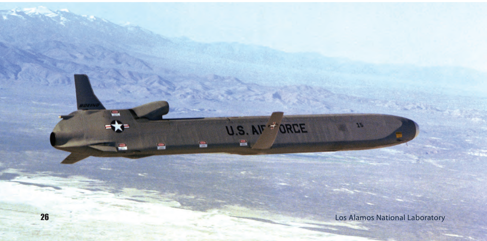
The AGM-86B is an air-launched cruise missile that can be launched from a B-52 Stratofortress and can be armed with a nuclear warhead. The AGM-86B was first built in 1977 with a life-expectancy to 2020 but the Air Force plans to extend its service life to 2030 or later. (Photo: U.S. Air Force)
